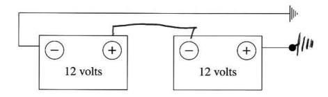
(e) In the diagram below, draw lines to show how to connect the terminals to **1** maintain battery output voltage at 12 volts.
